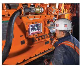
Serving as a type of interface between the operator and the machine, the custom display computer designed for Joy Global is constructed to operate in high ambient temperatures and withstand high vibration, shock, and moisture.
